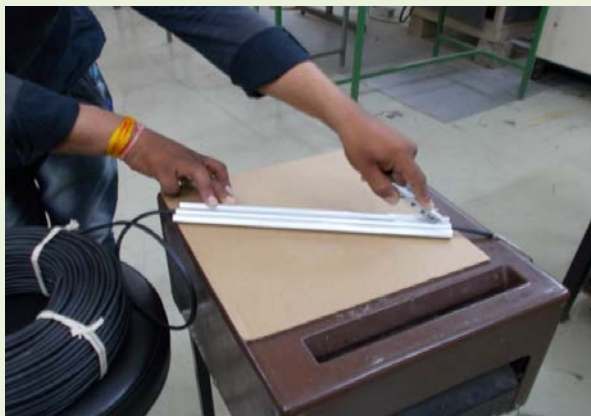
Fig. 34 Reuse of plastic sheath as protection jackets (1/2)
