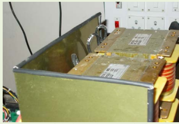
Fig. 35 Reuse of plastic sheath as protection jackets (2/2)
